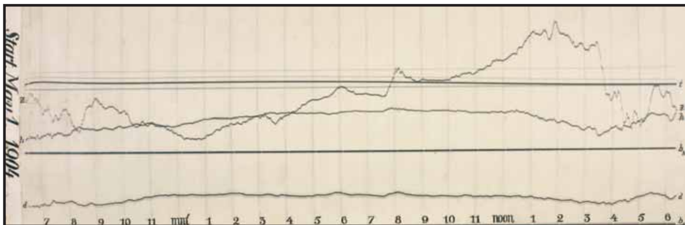
Automatic magnet readings from the Gjøa expedition. Photo NB
