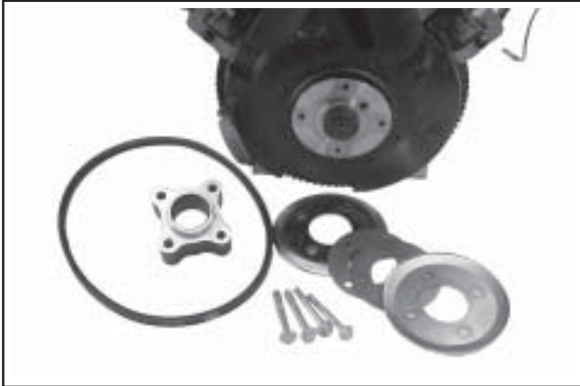
Figure 9-32. Disassembled Lower Pulley Assembly.
