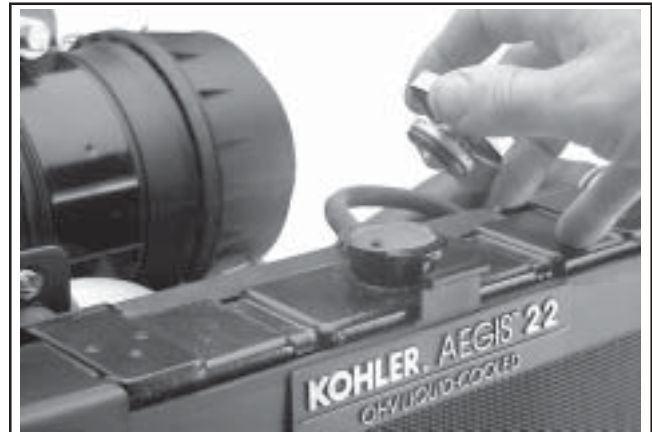
Figure 11-123. Radiator Cap (Install After Filling).
