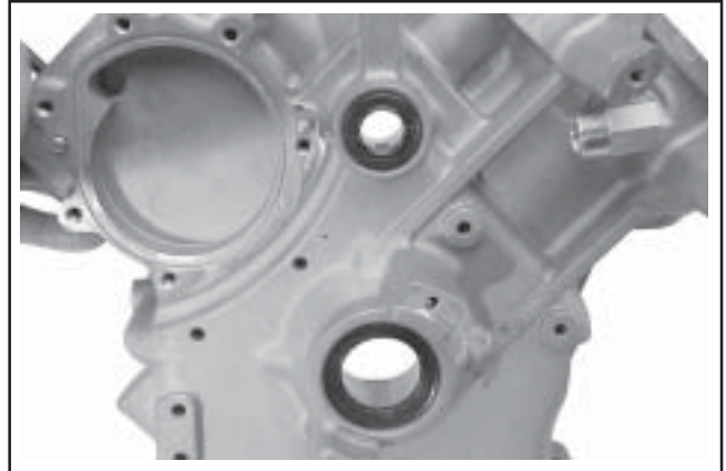
Figure 9-66. Oil Seals (Flywheel Side and Camshaft).
