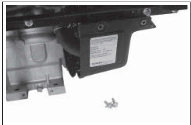
Figure 9-8. Removing Lower Flywheel Cover.
