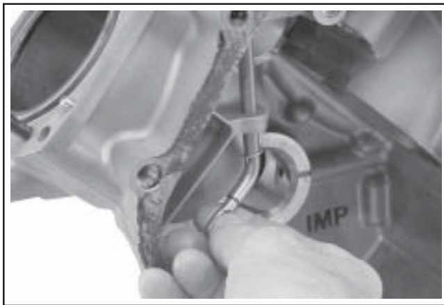
Figure 11-3. Installing Governor Shaft.
