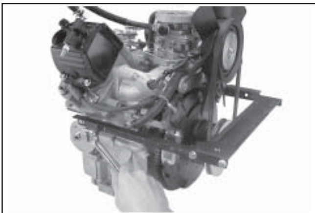
Figure 11-101. Mounting Lower Radiator Supports.
