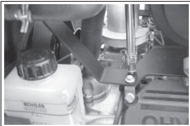
Figure 9-11. Remove Upper Radiator Support Screws.
