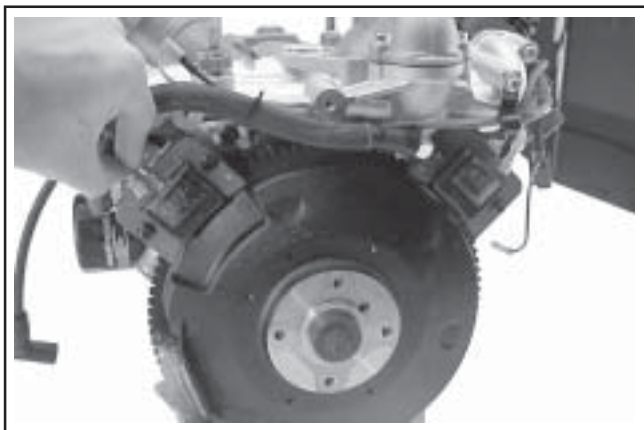
Figure 9-36. Removing Kill Leads from Ignition Modules.
