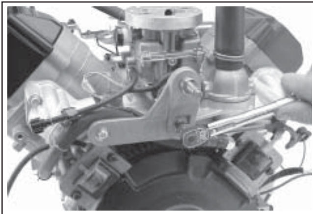
Figure 11-92. Installing Upper Pulley Bracket.
