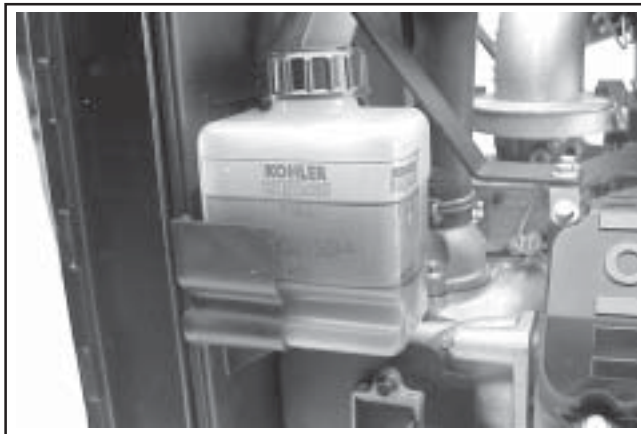
Figure 7-5. Coolant Levels on Reservoir.
