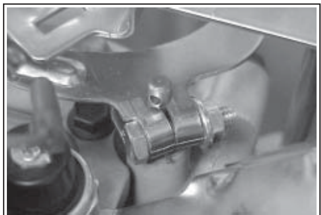
Figure 5B-33. Checking "Split" of Clamp.
