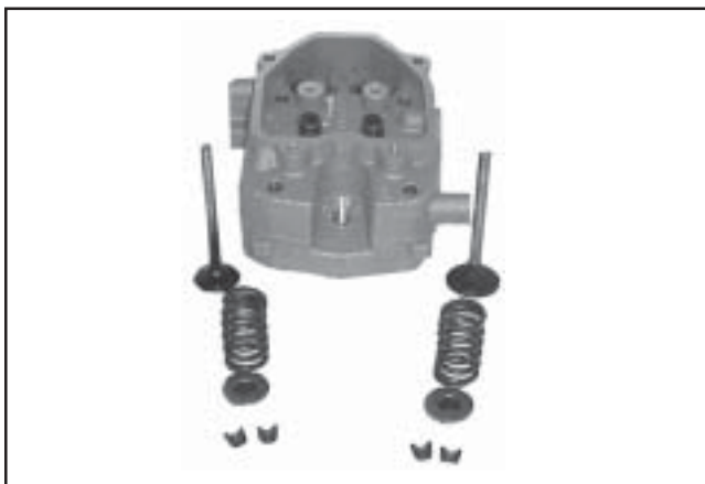
Figure 11-31. Disassembled Head and Valve Components.
