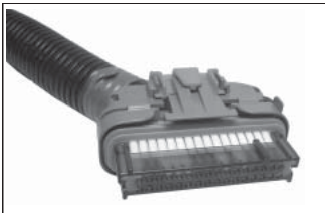
Figure 5B-19. “32 Pin” (MSE 1.1) Plastic-Cased ECU Connector.
