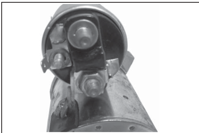
Figure 8-44. Positive (+) Brush Lead Connection.
