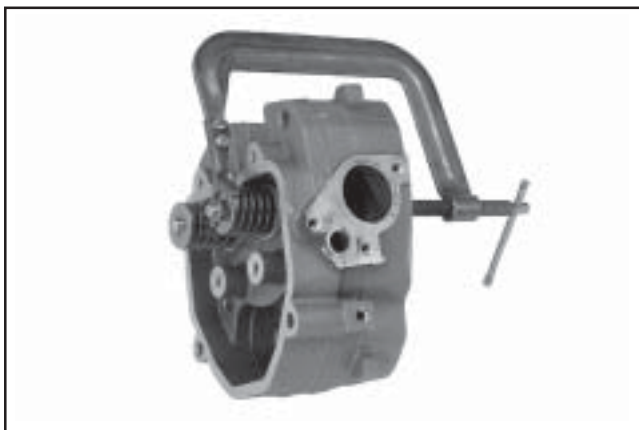
Figure 9-55. Compressing Valve Springs.
