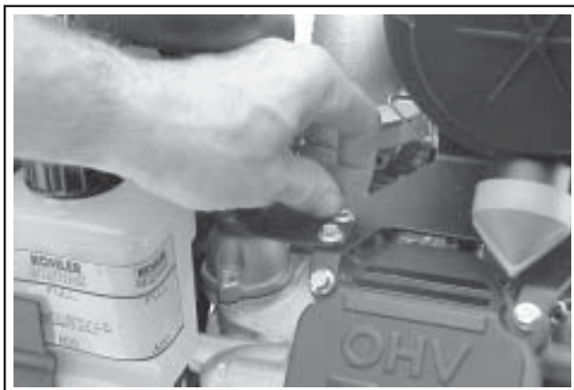
Figure 11-112. Installing Upper Support Screws.
