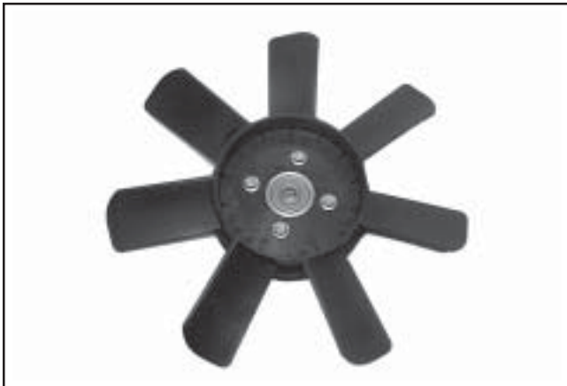
Figure 11-96. Fan Assembly (Rear View).
