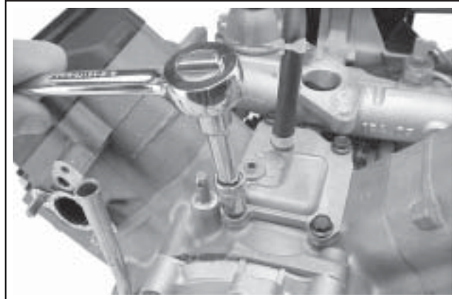
Figure 9-25. Removing the Breather Cover Screws.
