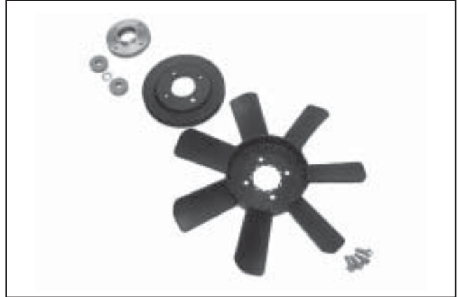
Figure 9-34. Disassembled Fan Assembly Component.
