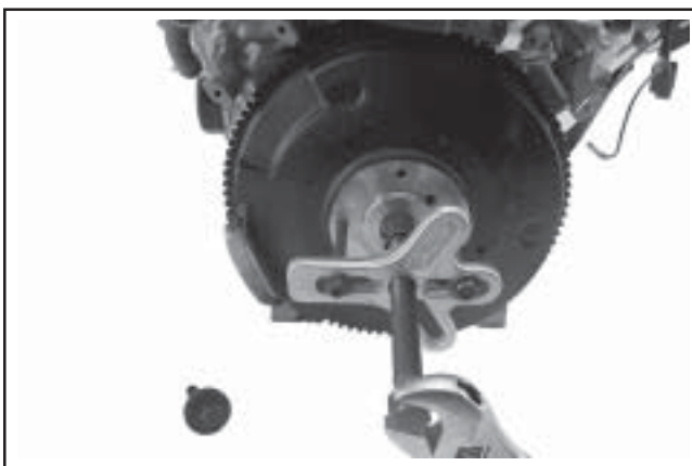
Figure 9-39. Removing Flywheel with Puller.
