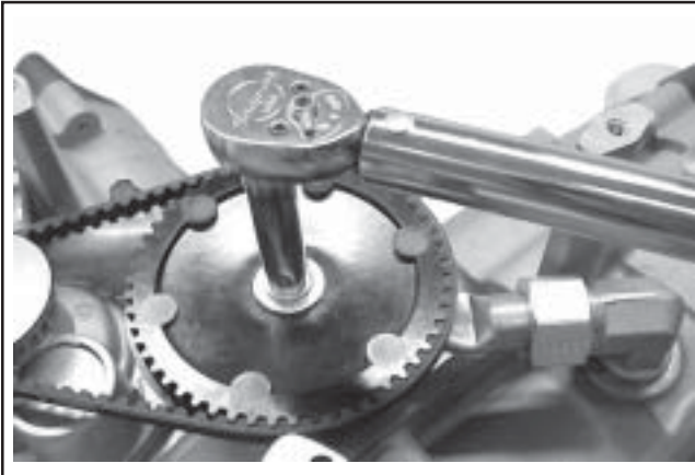
Figure 11-55. Torquing Mounting Screw of Cam Pulley.
