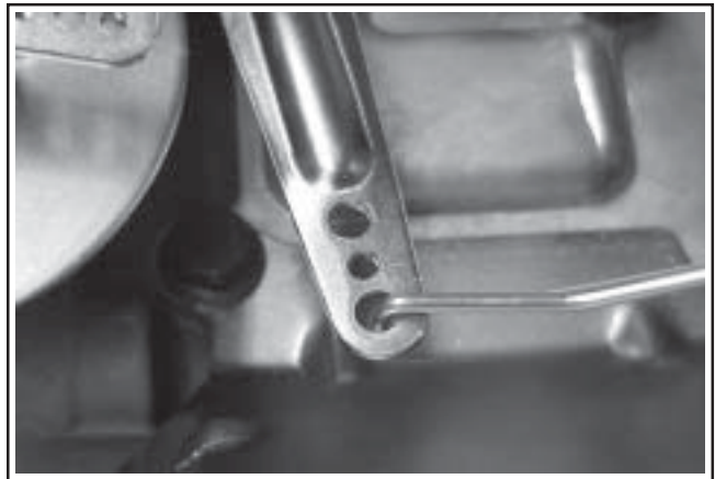
Figure 5B-32. Throttle Link in Center of Hole.
