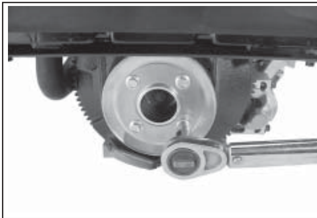
Figure 7-11. Torquing Lower Pulley Mounting Screws.
