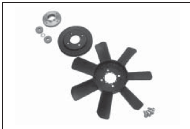
Figure 11-94. Fan Assembly Components - Disassembled Layout.
