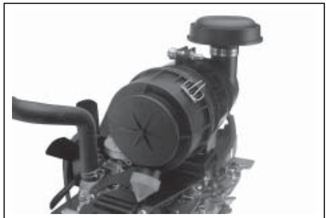
Figure 11-108. Dust Ejector Valve and Rain Cap Position.
