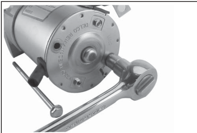
Figure 8-19. Removing Thru Bolts.
