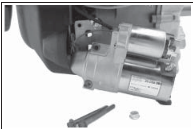
Figure 9-2. Removing Starter Assembly.
