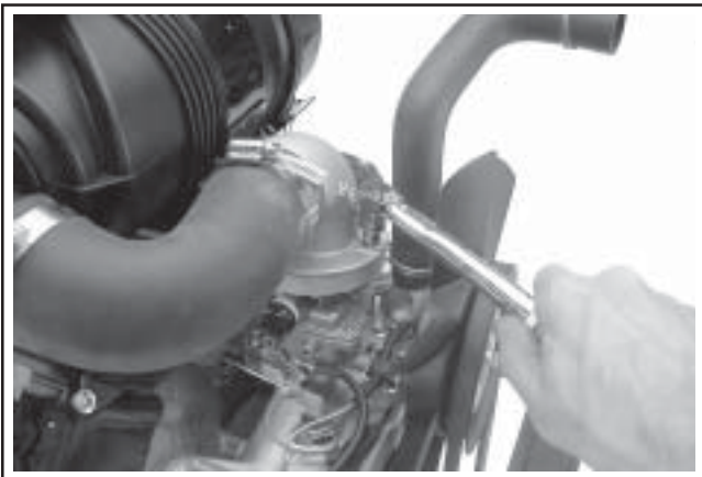
Figure 11-105. Torquing Elbow Mounting Screws.
