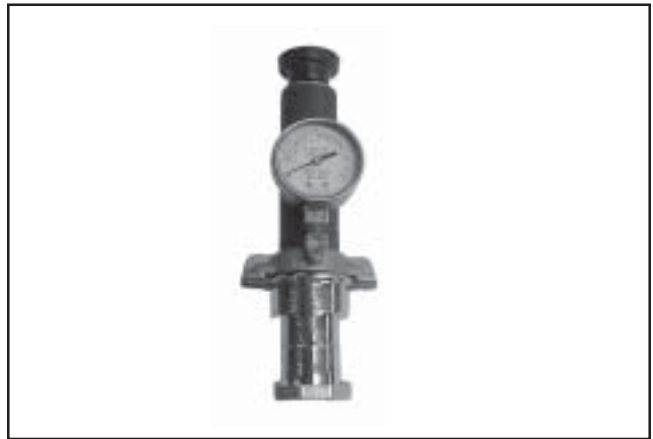
Figure 7-15. Adapter Installed onto the Tester.
