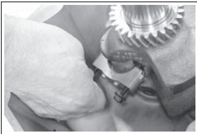
Figure 11-8. Attaching #1 Rod Cap.
