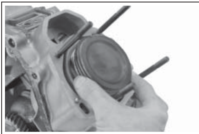
Figure 9-62. Removing Piston(s).
