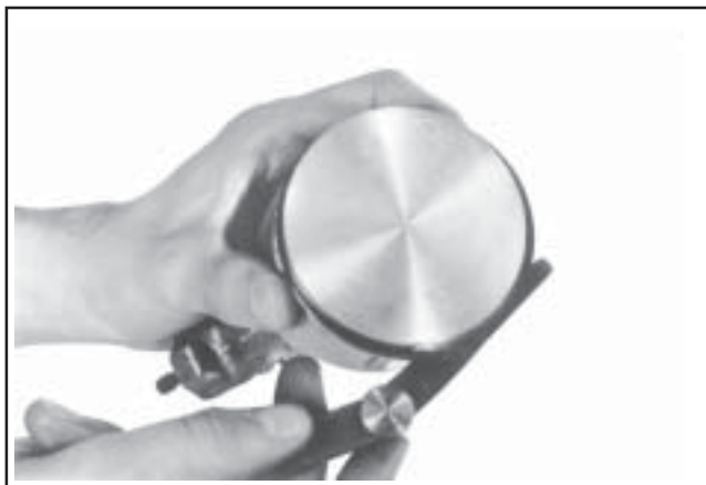
Figure 10-10. Measuring Piston Ring Side Clearance.
