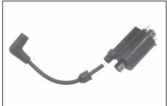
Figure 5B-18. Ignition Coil.
