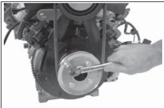
Figure 11-100. Torquing Lower Pulley Screws.
