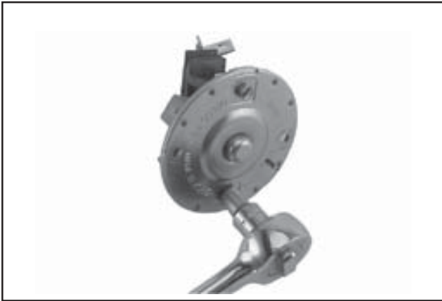
Figure 8-30. Removing Brush Holder.
