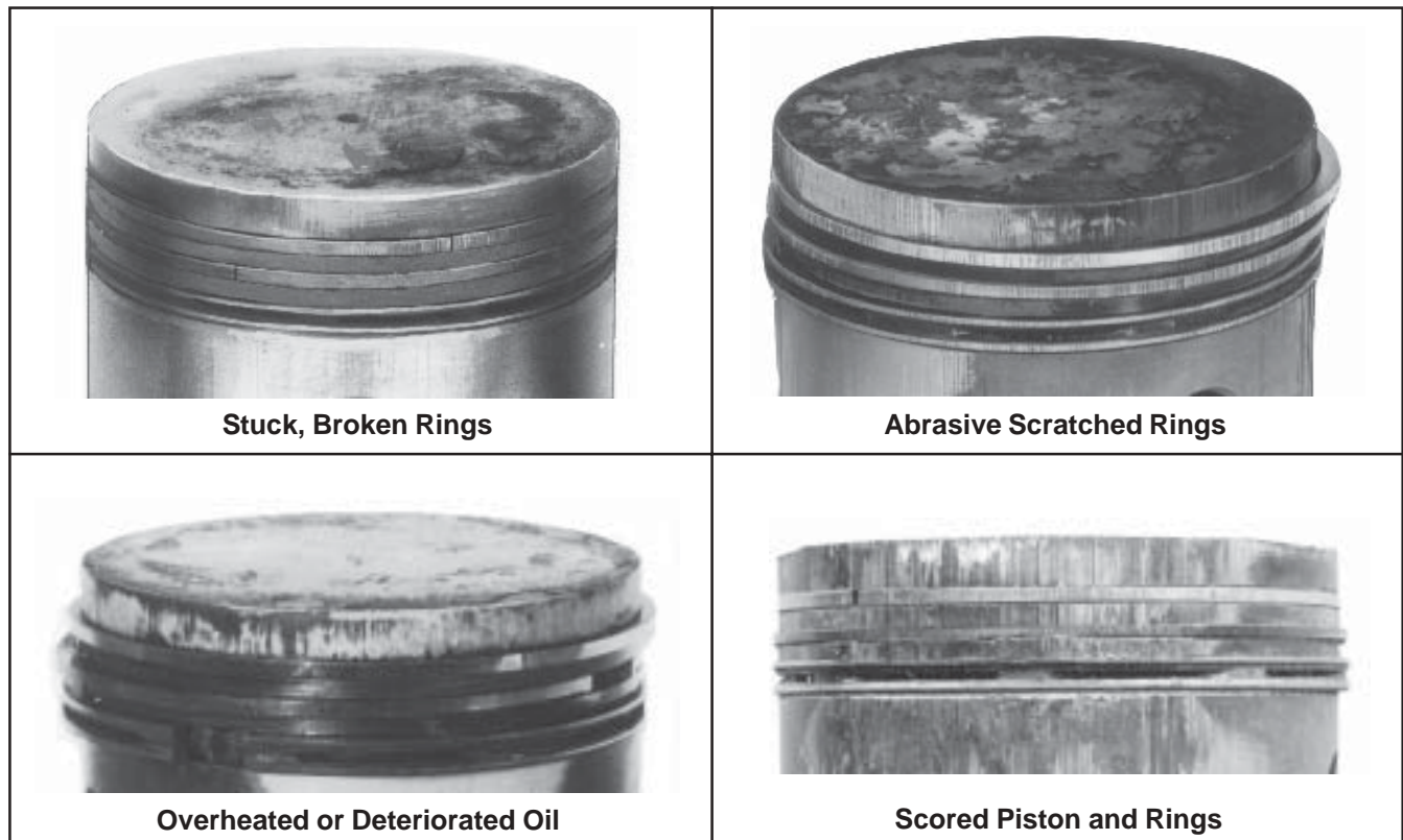
Figure 10-8. Common Types of Piston and Ring Damage.
