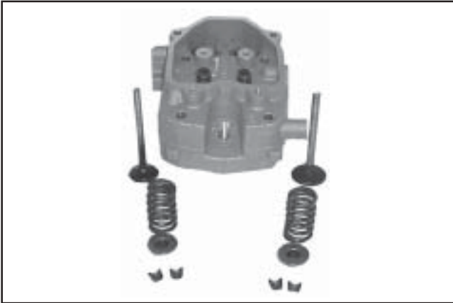
Figure 9-56. Disassembled Head and Valve Components.
