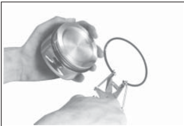
Figure 10-11. Installing Piston Rings With Expander.
