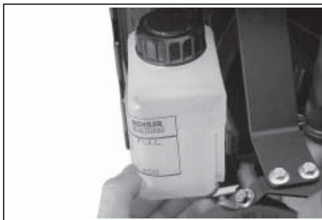
Figure 7-8. Removing Reservoir.
