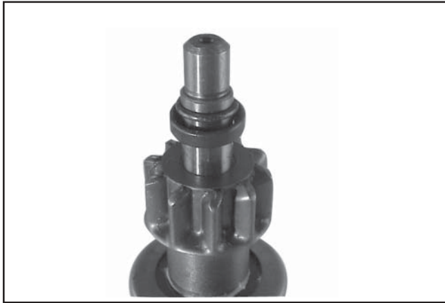
Figure 8-24. Retaining Ring Detail.
