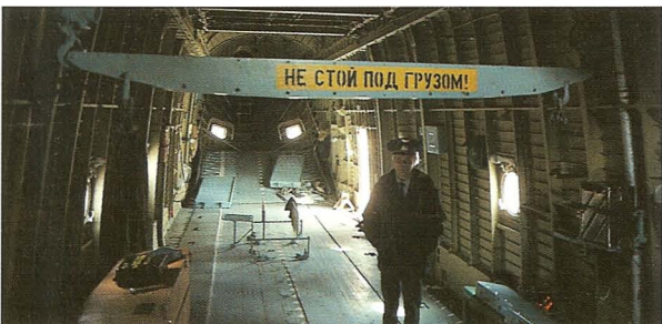
(Above) The two-ton capacity crane inside the Mil Mi-26, for heavy-duty in the oilfields of the Tyumen region.
