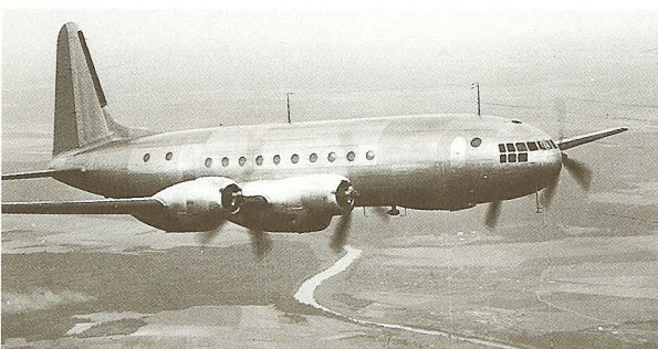
The Ilyushin 18, first flown on 30 July 1947, was a 60-seat four-engine airliner which never went into production. It was too large for the traffic of the day and demanded ground support which would not be available for years. (photo: Ilyushin Design Bureau)
