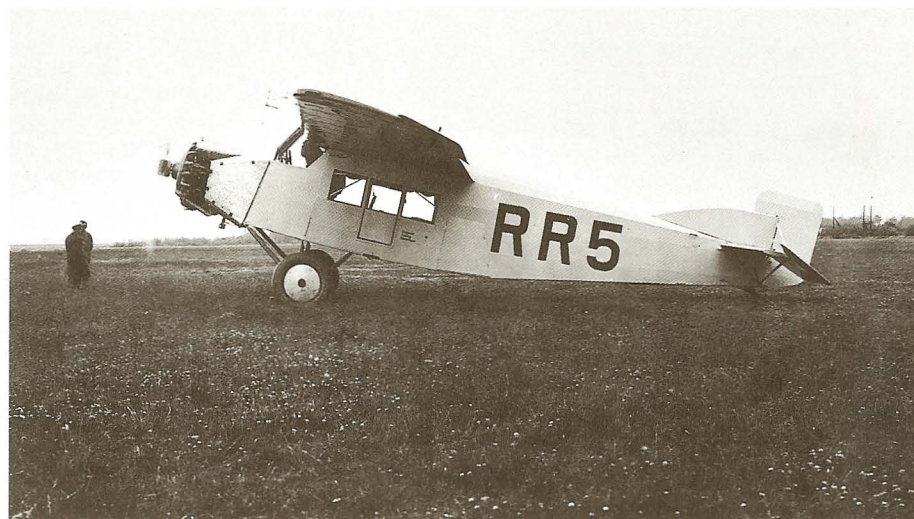
Fokker F.III RR 5 was converted by Deutscher Aero Lloyd at Berlin-Staaken (directed by technical manager Dr Ing Karl Grulich), with a revised fuselage, tail unit, cockpit, and landing gear, and — later — a Bristol Jupiter radial engine. In this guise, it was designated Grulich V1a. (photo: Lufthansa)
