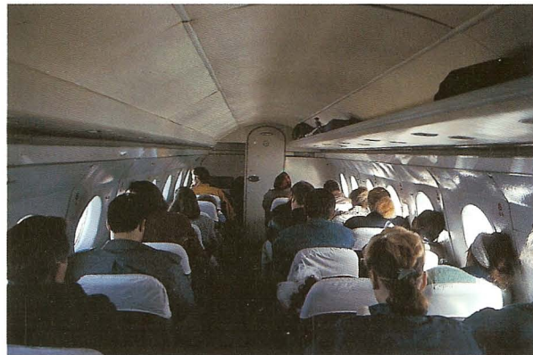
Cabin of a Yak-40 in 24-seat layout. In this version, baggage racks are open and on one side only. (Photos: R.E.G. Davies)
