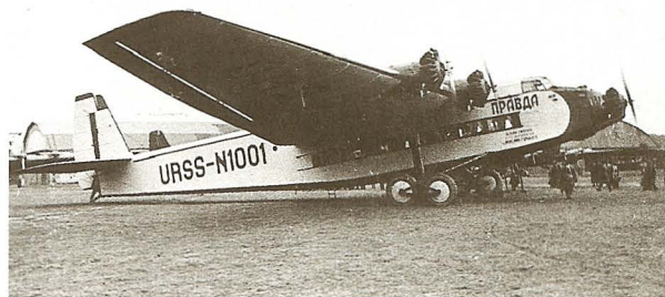
The only example of the ANT-14, and one of the few five-engined aircraft ever built. (photo: Boris Vdovienko)
