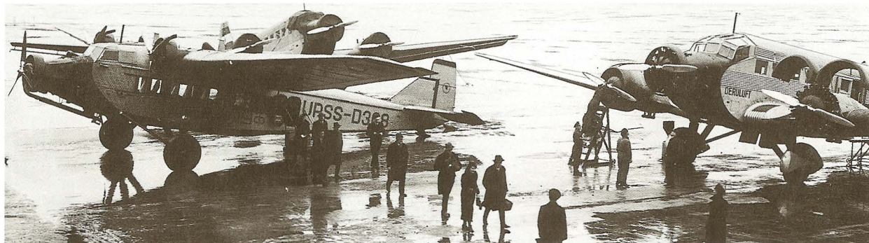
The ANT-9 and the Junkers-Ju 52/3m, both flying for Deruluft just before it stopped service, were representative of the generation of airliners that depended on corrugated metal for longitudinal stiffness. This picture was taken at Königsberg. (photo: Lufthansa)
