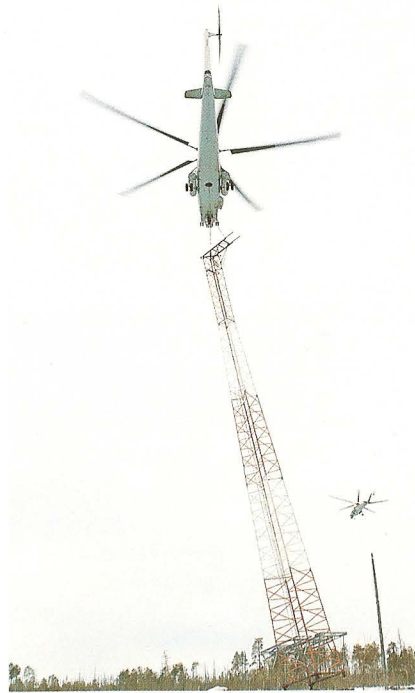
(Top right) A Kamov Ka-25K (SSSSR-21110). (J.M.G. Gradidge via John Stroud) (Right) A Mil Mi-10 transports an electricity transmission tower. A large percentage of the nationwide high-tension electricity powerline grid of the Soviet Union was constructed with the help of flying cranes. (V. Grebnev) (Top left) The Mil Mi-26T, developed from the Mi-6, with more powerful engines to drive and eight-bladed rotor, is the champion heavy-lifter, able to lift vertically a load of twenty tons. (R.E.G. Davies) (Bottom left) A Kamov Ka-26 (SSSR-19529) on ambulance duty. (V. Grebnev)
