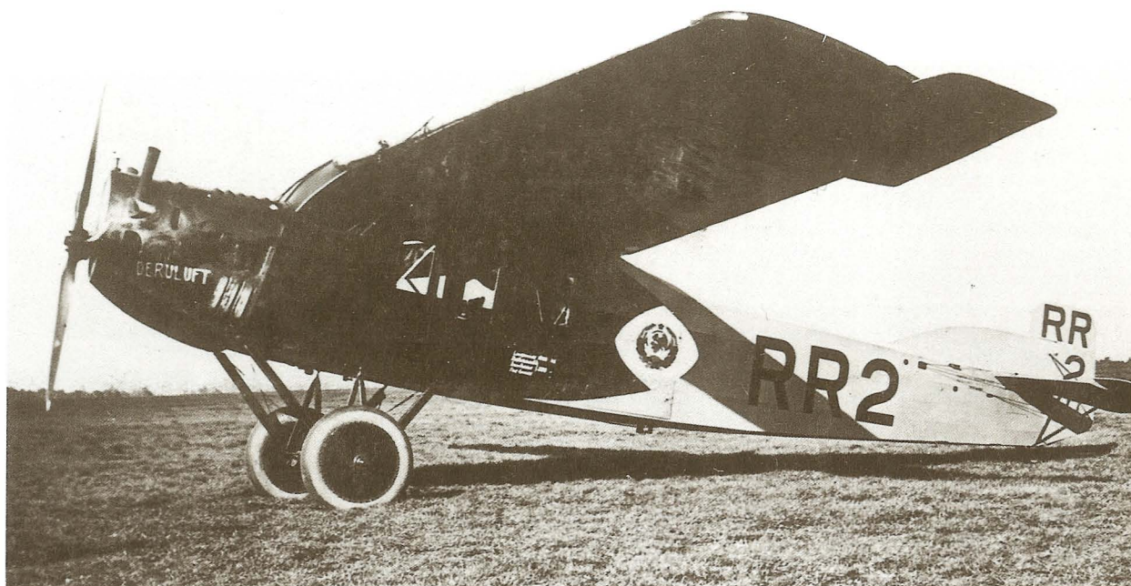
A Fokker F.III of Deruluft. The pilot was seated on the port side of the engine, in front of the passenger cabin. (photo: Lufthansa)
