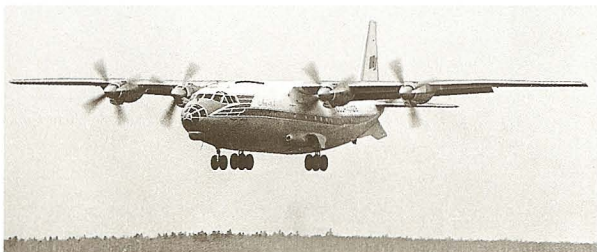
An-10A SSSR-11219 displays the definitive configuration with two vertical fins and no endplate tailplane fins. (Courtesy John Stroud)
