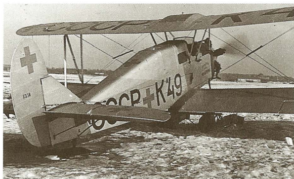
U-2S Sanitary Samolyet, or ambulance aeroplane (msn 6350).
