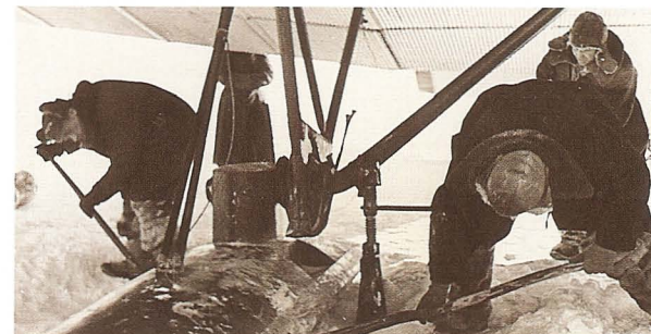
In the Arctic, aircraft frequently stuck in the snow when icing effectively glued them to the runway. Such scenes as this were familiar in the north. The aircraft is an ANT-7. (photo: Boris Vdovienko)
