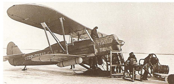
A Polikarpov U-2 (Po-2), diminutive maid-of-all-work, was to be seen everywhere during the War. This Aeroflot U-2 (SSSR-L3373) pictured at Tobolsk in 1941 has a sliding canopy enclosed cockpit for the pilot, and three passenger windows in the fuselage and containers underneath the wings. (photo: Boris Vdovienko)
