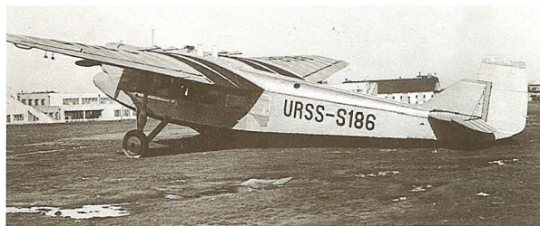
The twin-engined PS-9 was the main production version of the ANT-9. (photo: Boris Vdovienko)
