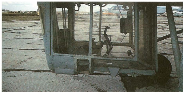
(Top) The supplementary control cabin of the giant Mil Mi-10. Rearward facing, the pilot has direct control of the helicopter, working in unison with the winch controller. (photos: R.E.G. Davies) (Bottom) This picture of the Kamov Ka-32 (with another hovering behind) illustrates the contrarotating rotorhead mechanism. (V. Grebnev)
