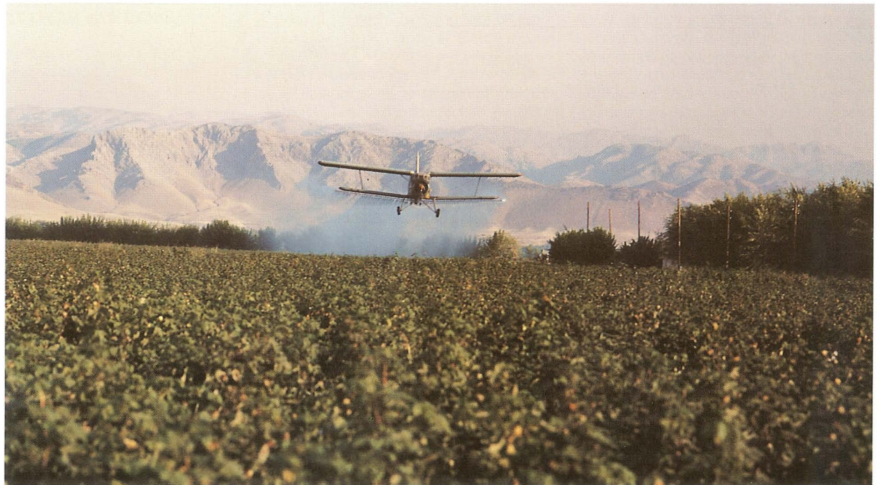
During the summer months, upwards of 2,500 Antonov An-2s are engaged in crop-dusting and -spraying, and other agricultural work throughout Russia and the former Soviet republics. This one is spraying cotton in Tajikistan. (V. Grebnev)
